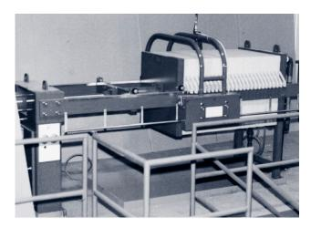
The flocs at the bottom of the decanter were pumped into the filter press. At that point, the percentage of solids increased from 3% to 5% for the sludge to about 45% to 55% in the filter press cake.
